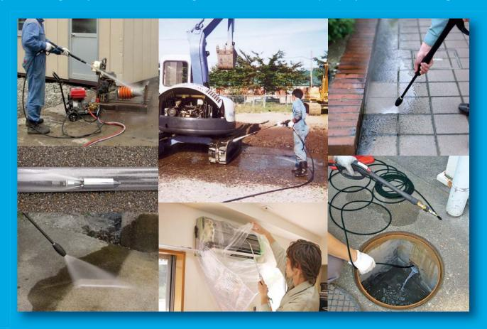
The second function is pipe cleaning. On some machines, the gun can be exchanged for a pipe cleaning hose. The pipe cleaning hose can run inside the pipe and wash away accumulated dirt with the impulse of jetting water.
