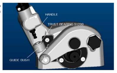
1 2 . Install Steel Ball 3/16 and then Hex Socket Set Bolt M6x15L(with Hex Nut M6) to the screw hole.
