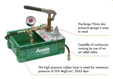
Either Hand operated or powered by a Rechargeable **Drill or Screwdriver**
